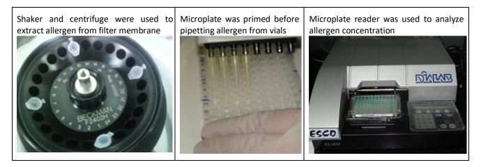
Operator protection efficiency was calculated by comparing the amount of allergen captured by the cassettes worn by the operator against the allergen sampled on top of dirty cages.
