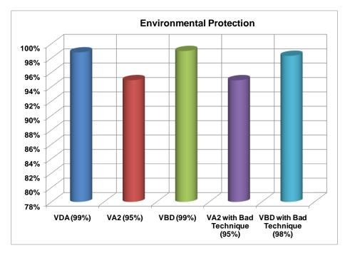
1. All three tested cabinets (VDA, VA2, VBD) have same high operator protection level of 99% when operated using good technique.
